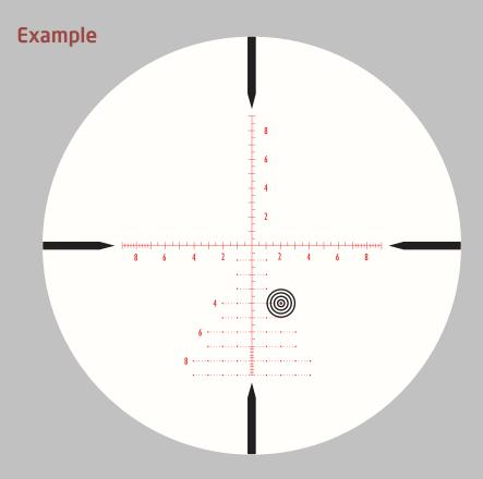
Use 4 mil drop line to compensate a 86.4 inch bullet drop at 600 yards, 2 mil wind correction for 15 mph wind from left to right.
