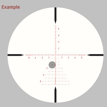
1 mil lead holdover for a moving target traveling left to right at 500 yards. Bullet flight time is 1 second during which the target traveled 1.5 feet. No wind.
