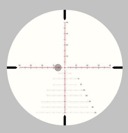
6 moa wind correction for 10 mph wind from right to left @ 600 yards. Elevation turret has been dialed up to compensate bullet drop, just simply use center horizontal cross line to holdover for wind correction
