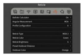
When the Athlon Ballistics APP is connected to the scope, go to the general settings to access the reticle settings.
