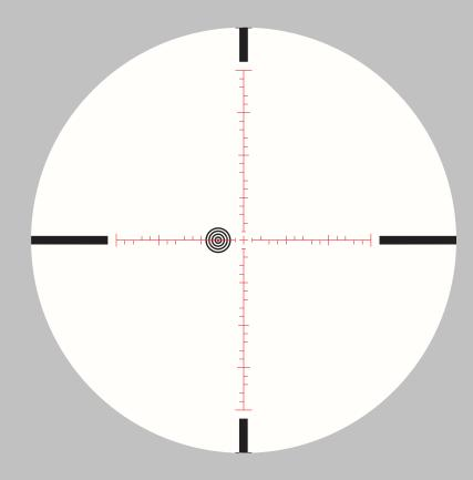
6 moa wind correction for 10 mph wind from right to left at 600 yards. Elevation turret has been dialed up to compensate bullet drop, just simply use center horizontal cross line to holdover for wind correction
