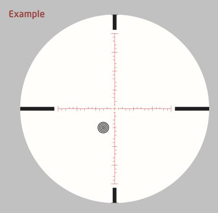
Use 10 moa for 60 inch bullet drop for a target at 600 yards, 6 moa wind correction for 10 mph wind from right to left.
