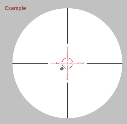
Use 10 moa for 60 inch bullet drop for a target at 600 yards, 10 moa wind correction for 20 mph wind from right to left.
