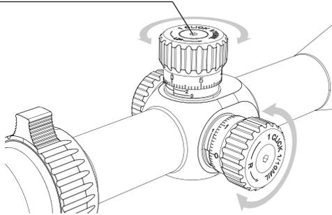
Athlon Argos BTR scopes have several options available, 1/2 MOA, 1/4 MOA, 1/5 MIL, and 1/10 MIL, for the click values of elevation and windage adjustment depending on different configurations of scopes and reticle selections. MOA, a unit of angular measurement, is defined as a minute of angle, a minute is 1/60th of one degree and 1/21600th of a circle. One MOA
