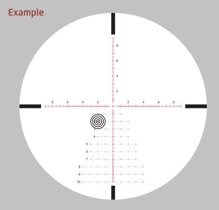
Use 3 mil to compensate a 54 inch bullet drop for a target at 500 yards, 2 mil wind correction for 15 mph wind from right to left.
