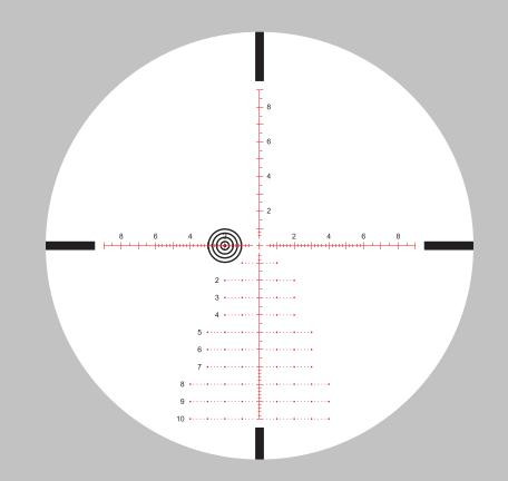
2 mil wind correction for 15 mph wind from right to left at 500 yards. Elevation turret has been dialed up to compensate bullet drop, just simply use center horizontal cross line to holdover for wind correction
