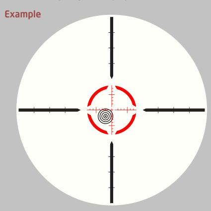
2 mil lead holdover for a moving target traveling from left to right at 300 yards (21.6 inch drop). Bullet flight time is 1 second during which the target traveled 3.6 feet. No wind.
