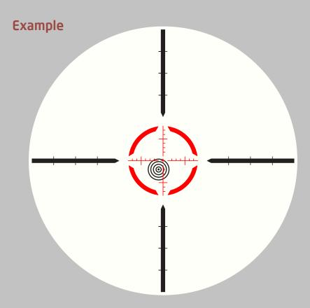
Use 2 mil to compensate a 21.6 inch bullet drop for a target at 300 yards, 1 mil wind correction for 15 mph wind from right to left.
