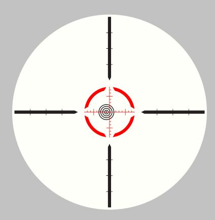
1 mil wind correction for 15 mph wind from right to left at 300 yards. Elevation turret has been dialed up to compensate bullet drop, just simply use center horizontal cross line to holdover for wind correction
