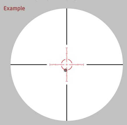
2 moa lead holdover for a moving target traveling at 2 mph from left to right at 600 yards. Bullet flight time is 1 second during which the target traveled 1 foot. No wind.
