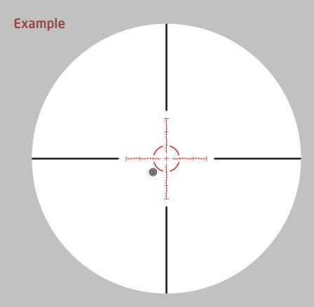
Use 10 moa for 60 inch bullet drop for a target at 600 yards, 10 moa wind correction for 20 mph wind from right to left.
