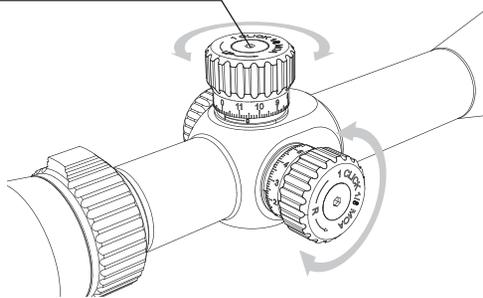
Athlon Argos BTR 10-40x56 scopes have 1/8 MOA for the click value of elevation and windage adjustment. MOA, a unit of angular measurement, is defined as a minute of angle, a minute is 1/60th of one degree and 1/21600th of a circle. One MOA equals 1.047-inch (rounded down to one inch) at 100 yards,
