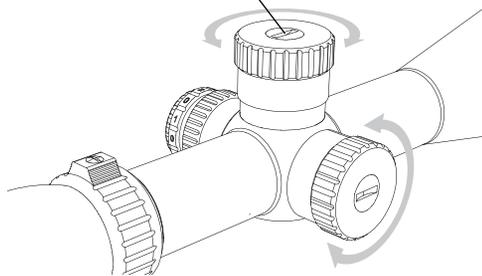
Athlon Midas BTR GEN2 scopes have several options available, 1/4 MOA, and 1/10 MIL for the click values of elevation and windage adjustment depending on different configurations of scopes and reticle selections. MOA, a unit of angular measurement, is defined as a minute of angle, a minute is 1/60th of one
