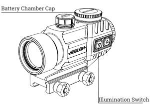
The illumination is powered by a lithium CR2032 3V battery. Remove the battery chamber cap by turning it counter-clockwise and then set the battery with the positive (+) side facing up. Reinstall the cap by turning it clockwise, DO NOT OVER TIGHTEN.
