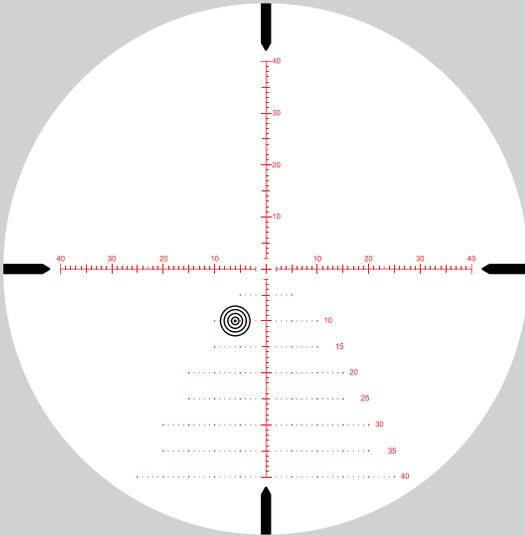
*Use 10 moa for 60 inch bullet drop for a target @ 600 yards, 6 moa wind correction for 10 mph wind from right to left.*
