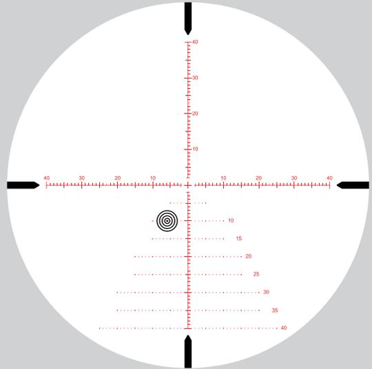
*5.9 moa lead holdover for a moving target traveling at 2 mph from left to right at 600 yards. Bullet flight time is 1 second during which the target traveled 2.94 feet. No wind.*
