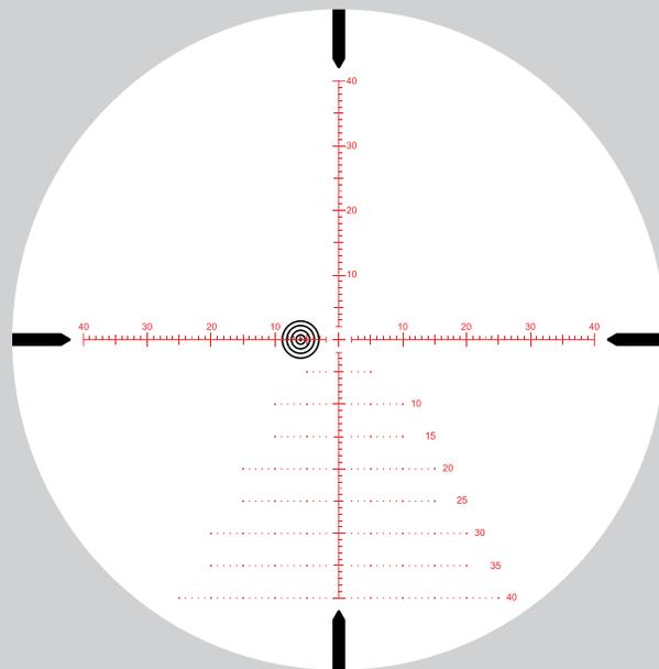
*6 moa wind correction for 10 mph wind from right to left @ 600 yards. Elevation turret has been dialed up to compensate bullet drop, just simply use center horizontal cross line to holdover for wind correction*
