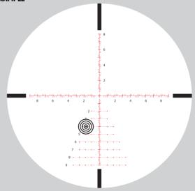
1.95 mil lead holdover for a moving target traveling at 2 mph from left to right @ 600 yards. Bullet flight time is 1 second during which the target traveled 2.94 feet. No wind.
