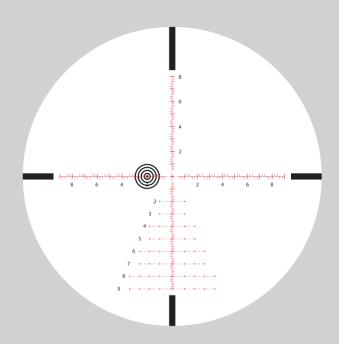
2 mil wind correction for 15 mph wind from right to left at 500 yards. Elevation turret has been dialed up to compensate bullet drop, just simply use center horizontal cross line to holdover for wind correction.
