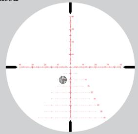
5.9 moa lead holdover for a moving target traveling at 2 mph from left to right at 600 yards. Bullet flight time is 1 second during which the target traveled 2.94 feet. No wind.
