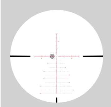
6 moa wind correction for 10 mph wind from right to left @ 600 yards. Elevation turret has been dialed up to compensate bullet drop, just simply use center horizontal cross line to holdover for wind correction
