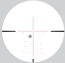
Use 10 moa for 60 inch bullet drop for a target @ 600 yards, 6 moa wind correction for 10 mph wind from right to left.
