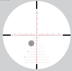
1.95 mil lead holdover for a moving target traveling at 2 mph from left to right at 500 yards. Bullet flight time is 1 second during which the target traveled 2.94 feet. No wind.
