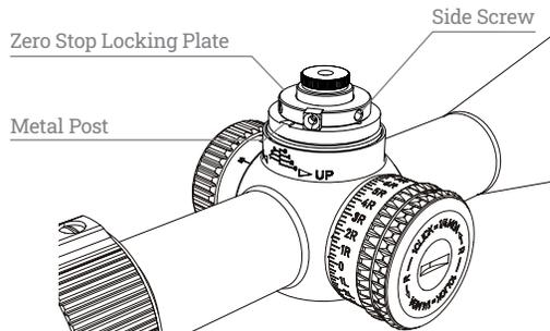
By zeroing the rifle at 100 yards, the shooter can calculate how many clicks of adjustment are needed for different distances or wind conditions. After shooting, the shooter can quickly turn the elevation knob clockwise (down direction) and go back to the zero position once the knob cannot be turned any further. **DO NOT OVERTURN THE ELEVATION KNOB ONCE IT STOPPED.**
