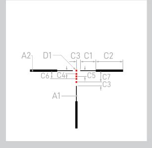
The MOA #05 reticle is a bullet drop compensation reticle specifically designed for 5.56 mm NATO /.223 REM round. The holdovers for bullet drop are extended to 200, 300, 400, 500, and 600 yards.
