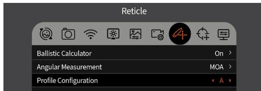
**Zero Setting:** 50, 100, and 200 Yard or Meter are available to choose from in the menu. Use the one shot zeroing feature in the menu to sight in. After zero is set, use the menu to select the preset zero distance under each profile. Please refer to Quick User Guide or User Manual on the product web page for detailed one shot zeroing instructions.
