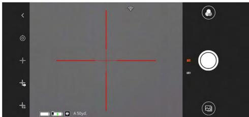
**Profile Configuration:** Letters A to J are assigned to 10 different profiles. The zeroing distance, zeroing location, reticle type, reticle color and reticle brightness are saved for each profile.
