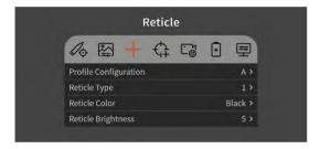
When the Athlon Ballistics APP is connected to the scope, go to the general settings to access the reticle settings.
